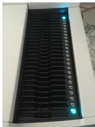
**Note: Do not load empty slide holders (i.e., without slides) into the SureScan scanner!**
